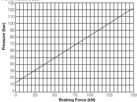
Braking force assumes a coefficient of friction between brake pad and brake disc of 0.4.
